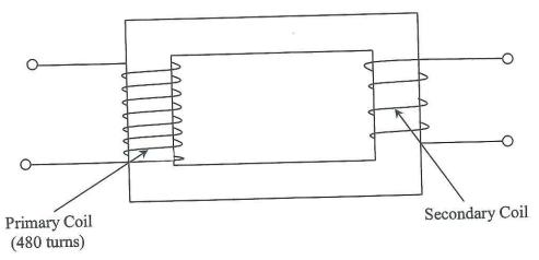
Using the information above, calculate the number of turns on the secondary coil. (1 mark)
