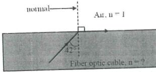
Use the information provided in the diagram to find the refractive index of the fiber optic material used. (1 mark)
