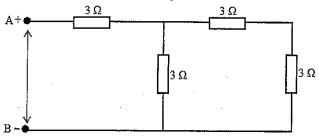
(i) Calculate the total resistance between points A and B.
