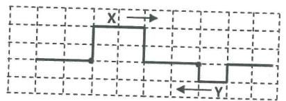
Identify the shape of the resultant wave after 2 seconds?
